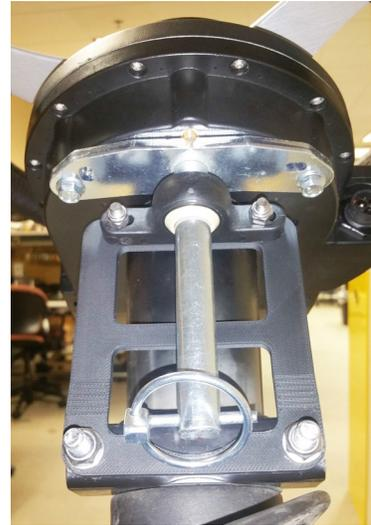
2. Insert the linchpin through the hole at the bottom of the t-bar (above right).
