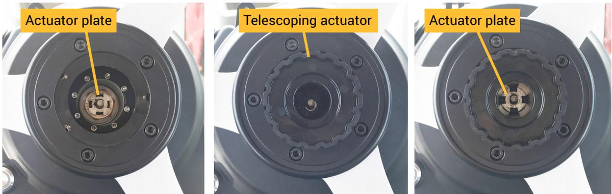
6. Snap the center cap (that came with the telescoping actuator parts) into the steering wheel cover.
