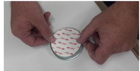
3. Position the mounting plate and press down hard for proper adhesion. When determining the location of the mounting plate, ensure that when you mount the antenna on the plate (next step) the antenna will be on the vehicle's centerline and pivot line.
