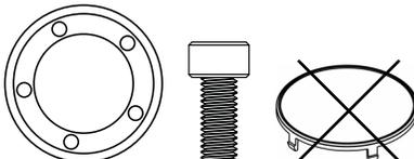
Steering wheel cover, socket head cap screws (5), and center cap (cap not used; use cap that comes with telescoping actuator instead)
