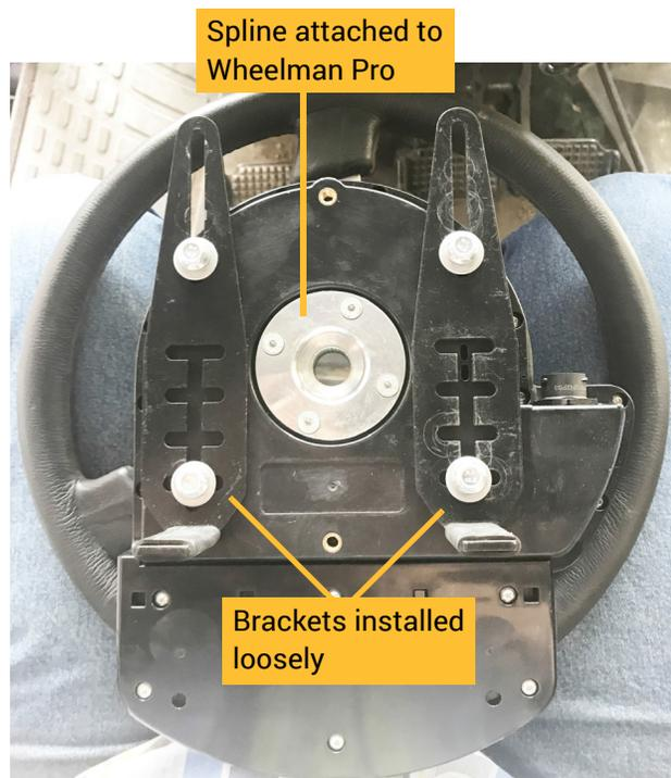
2. On the top side of the Wheelman Pro, install the new steering wheel (below left) and the steering wheel cover (below right)—although the photos below show the Wheelman already placed on the steering column, you may assemble these components on a flat surface, such as a workbench, before installing the assembly on the steering column. If you want to assemble these components while installing Wheelman on the steering column, complete step b below (removing the existing steering wheel) first.
