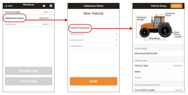
Starting on the Wheelman screen (see above left) tap Calibration Status, then on the Calibration Status screen (see above middle) tap Vehicle Dimension to display the Vehicle Setup screen.
