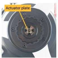
6. Snap the center cap (that came with the telescoping actuator parts) into the steering wheel cover.
