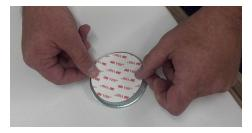
Position the mounting plate and press down hard for proper adhesion. When determining the location of the mounting plate, ensure that when you mount the antenna on the plate (next step) the antenna will be on the vehicle's centerline and pivot line.
