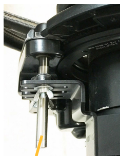
Pin through flange then into Flex
